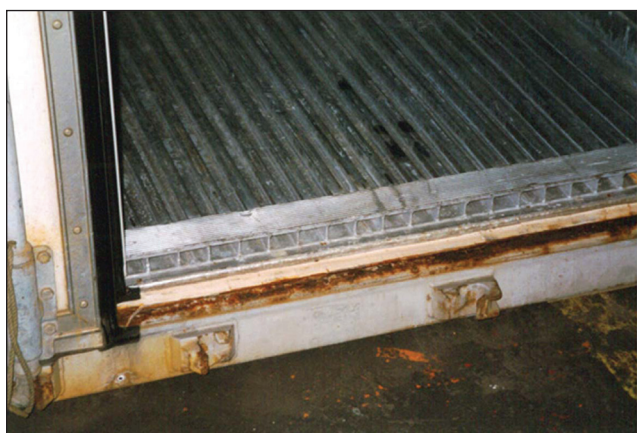
Figure 2 Floor refrigerated container [6] Slika 2. Rashladni kontejner s hladnim dnom
