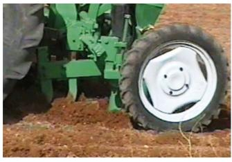
Figure 2. Mulch injection into soil by the machine
