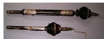
Figure 12 Axle-shaft with a groove and measuring devices for the torque measurement
