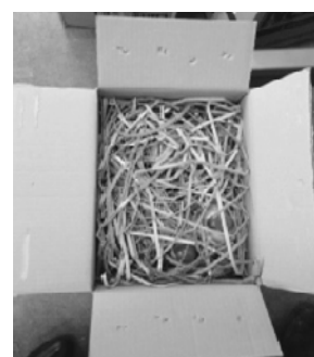
Figure 5. Cardboard strips made by cutting up incoming secondary packages and used as accessories
