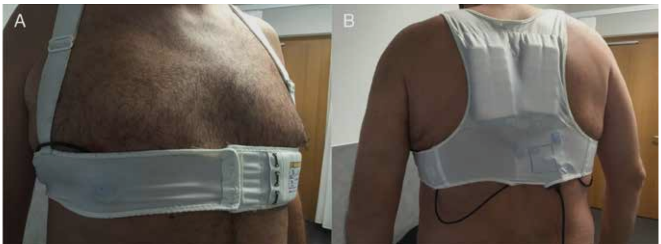
FIGURE 2. Wearable cardioverter defibrillator. Model of a wearable cardioverter defibrillator (images courtesy of J.S., reprinted with kind permission and patient consent).
