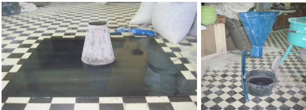
Figure 1 Disposition of the slump flow test (left) and V-funnel test (right) [12]
