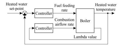
Figure 2. Standard PID control circuit used in full-scale
