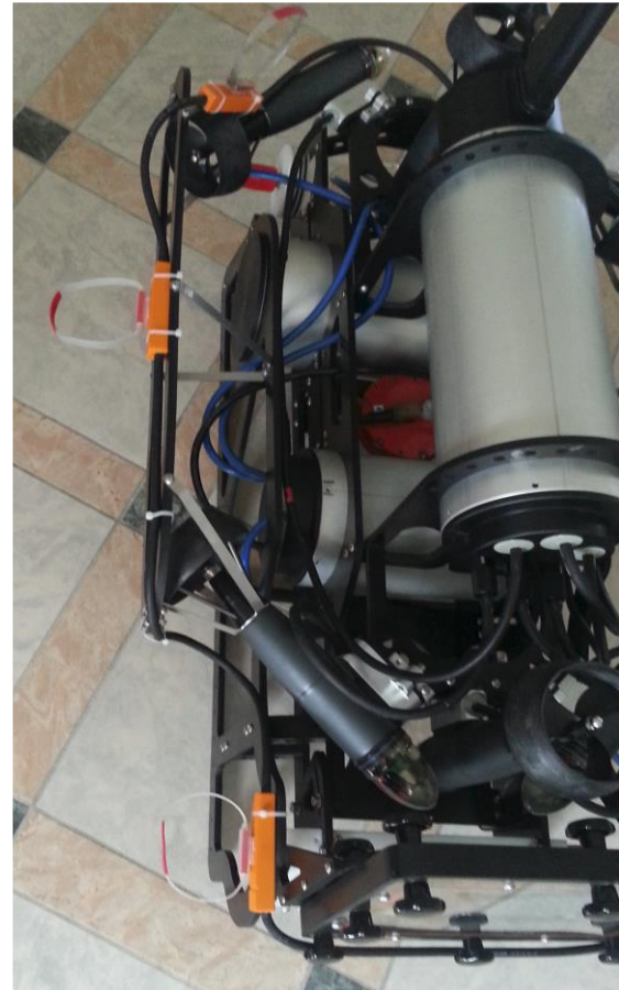
Figure 14 Magnetic kill switches installed on AUV
