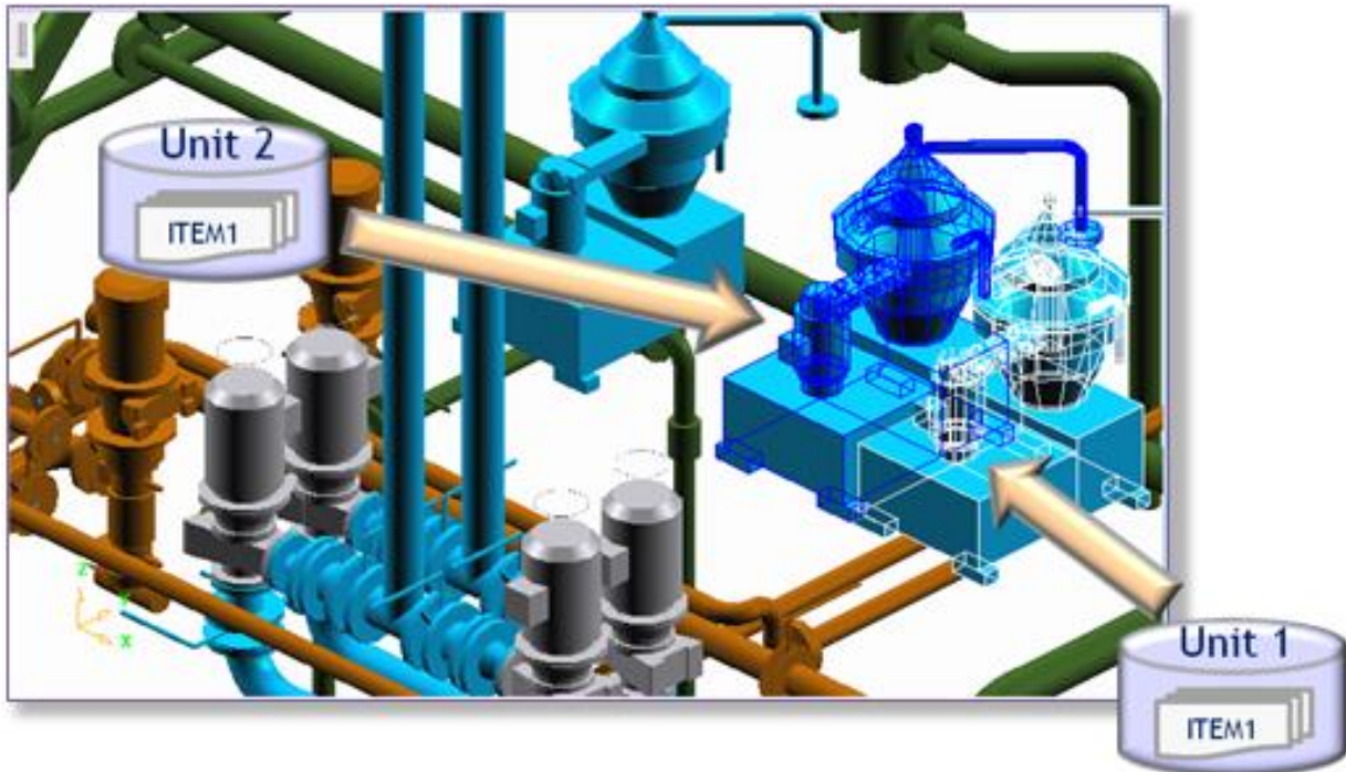
Fig. 10 Visual differences between an item in two series ship units
