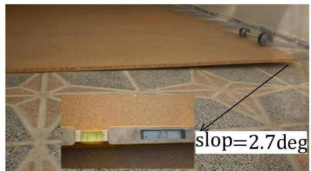
Fig. 10. Experimental setup with an object and surface with slope  $2.7^\circ$
