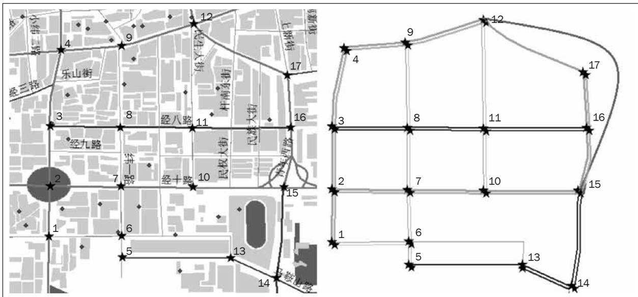
Figure 1 - Simulated Road Network Topology
