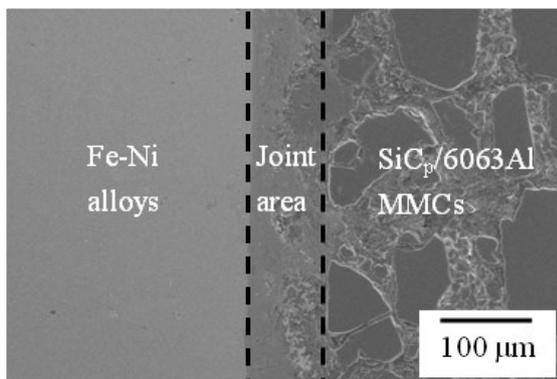
Figure 2. SEM image of the joint with soaking time of 30 min at 580 °C.
