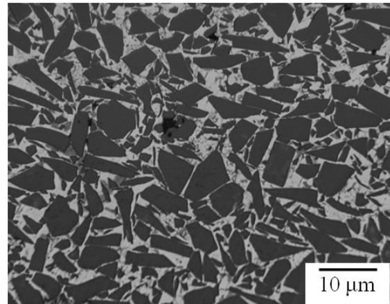
Figure 1. Microstructure of SiC<sub>p</sub>/6063Al MMCs with 55% volume fraction.
