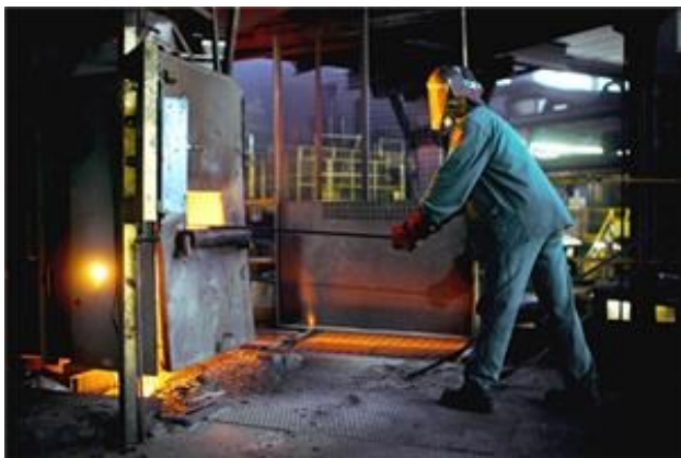
Figure 5. Production of specimens by sand casting: withdrawing a sample for tests on the molten metal.
