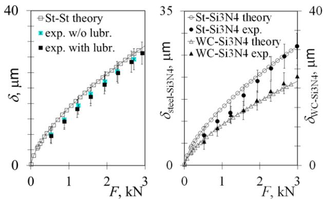
Figure 8. Theoretical and experimental values of interpenetration distances  $\delta$ .
