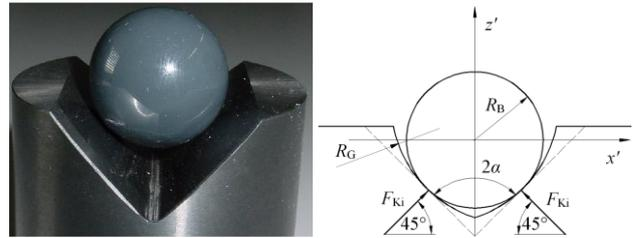
Figure 2. Ball – V-groove interface.
