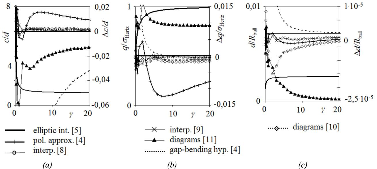
Figure 6. Ratio of the semi-axes lengths of the elliptical contact area (a), normalized contact stresses (b) and normalized interpenetration distances (c) versus the ratio of the radii of curvature  $\gamma$ .
