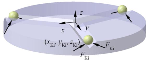
Figure 3. Information required to define a three V-groove kinematic coupling.
