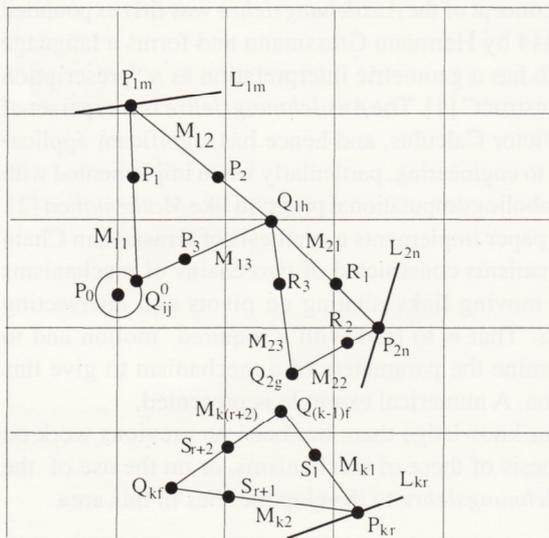
Figure 1: The Construction Scheme of Grassmann Chain Mechanism in the General Case
