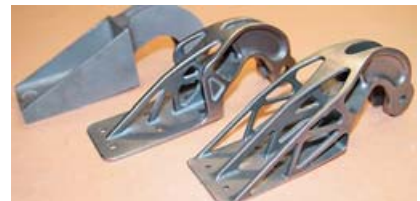
Fig.12 3D printed A320 hinges [17]
