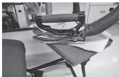
Fig.6 Placing felt under the iron base
