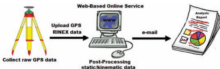
Figure 1: The basic working principle of web-based online services
