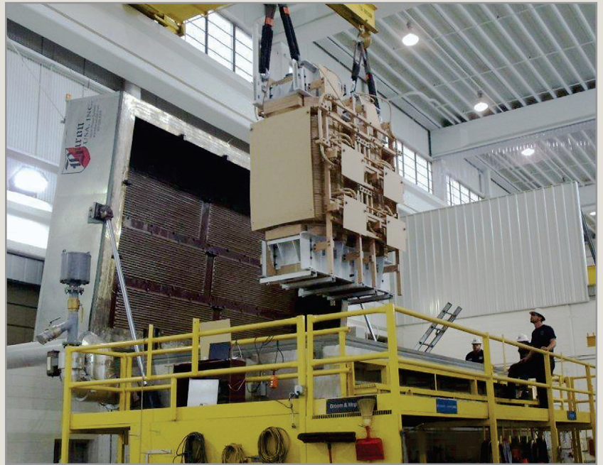
Figure 8: Top loading clamshell chamber
