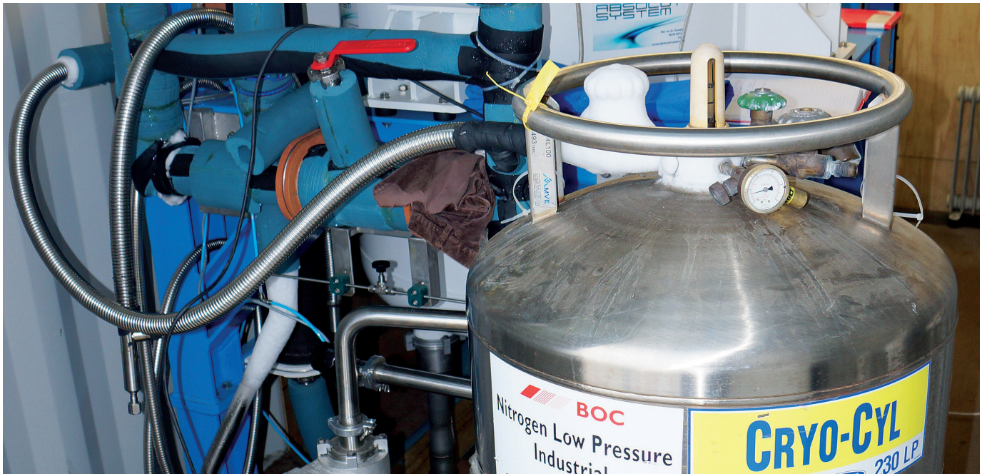
Figure 3. Cooling system for 1 MVA HTS transformer
