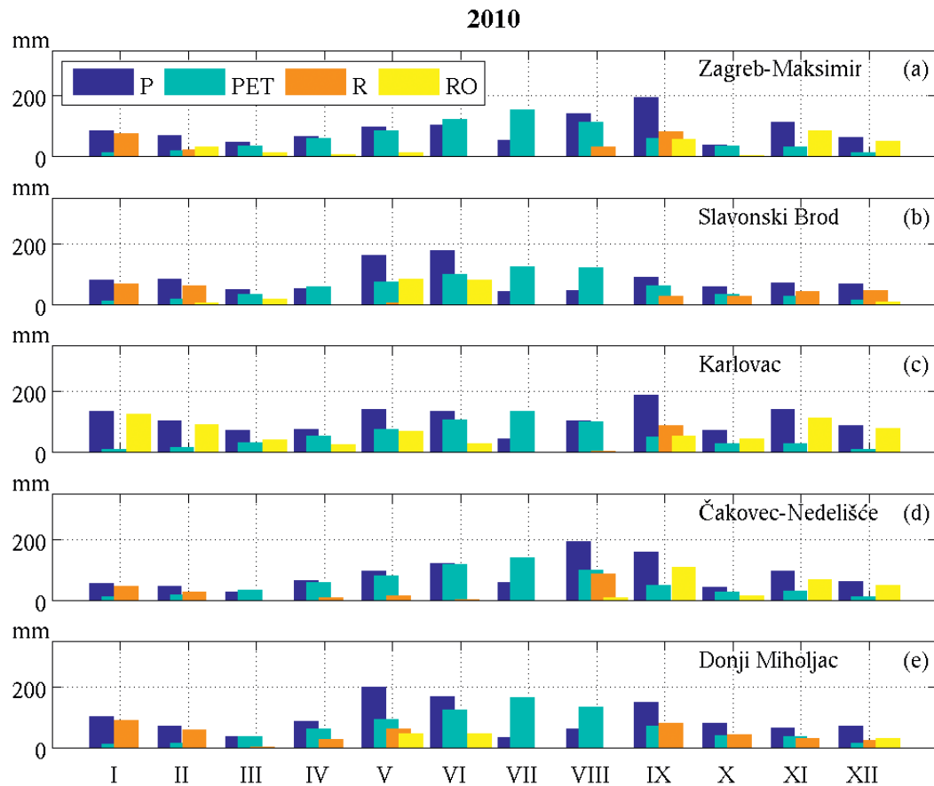
Figure 2. Water balance components in 2010 at 5 observed meteorological stations. P is precipitation, PET is potential evapotranspiration, R is groundwater recharge and RO is surface runoff.
