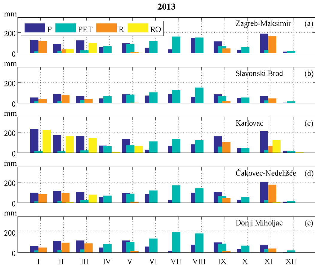
Figure 3. Water balance components in 2013 at 5 observed meteorological stations. P is precipitation, PET is potential evapotranspiration, R is groundwater recharge and RO is surface runoff.
