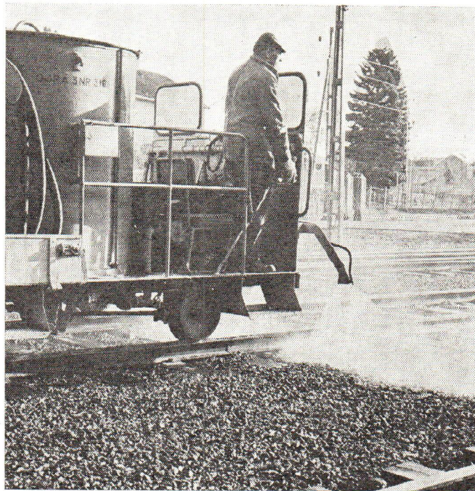
Fig. 1. The type of aggregate used for spraying herbicides on Swedish railways
