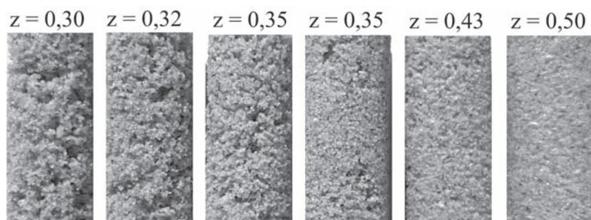
Figure 3 Side surfaces of cylindrical samples of sandmix O145 (z - compaction degree)
