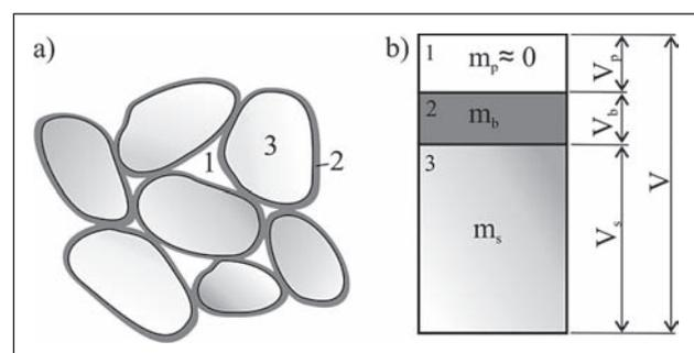
**Figure 1** Schematic presentation of three-phase structure of moulding sand (a) 1 – gaseous phase (air), 2 – liquid phase (binder), 3 – solid phase (sand); (b) volumetric fractions of individual phases
