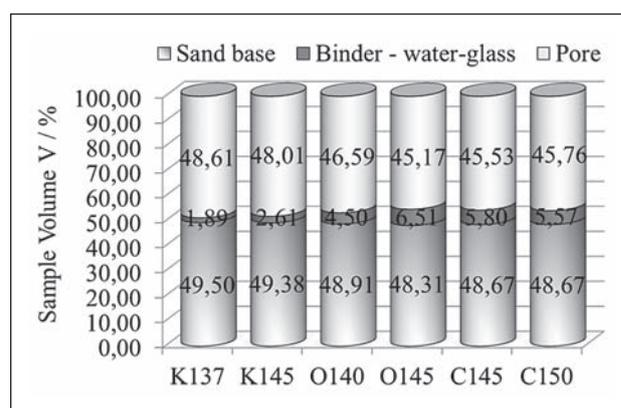
Figure 5 Volumetric percentage of individual phases in a cylindrical sample of moulding sand with volume  $8,44 \cdot 10^{-6} \text{ m}^3$  at compaction degree 0,5
