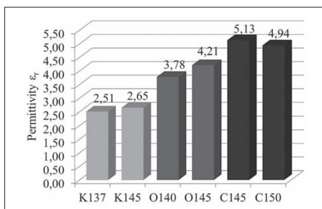
Figure 4 Relative permittivity of samples with compaction degree 0,5
