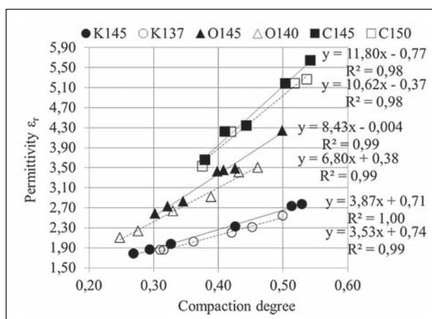
Figure 2 Relationship between permittivity and compaction degree of moulding sands
