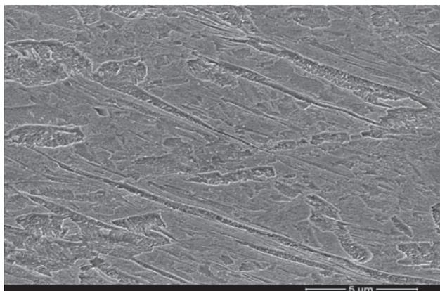
**Figure 1** Micrograph of PREMOMET® steel as initial condition.
