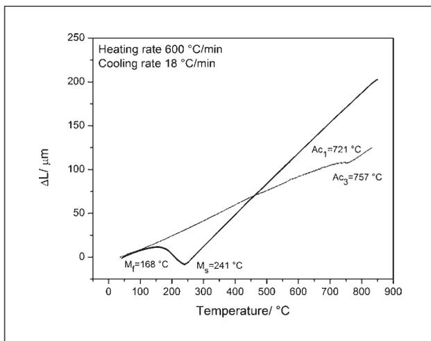
**Figure 5** Experimental dilatometric curve of PREMOMET® steel heated at 600 °C/min.
