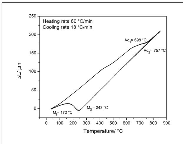
**Figure 4** Experimental dilatometric curve of PREMOMET® steel heated at 60 °C/min.
