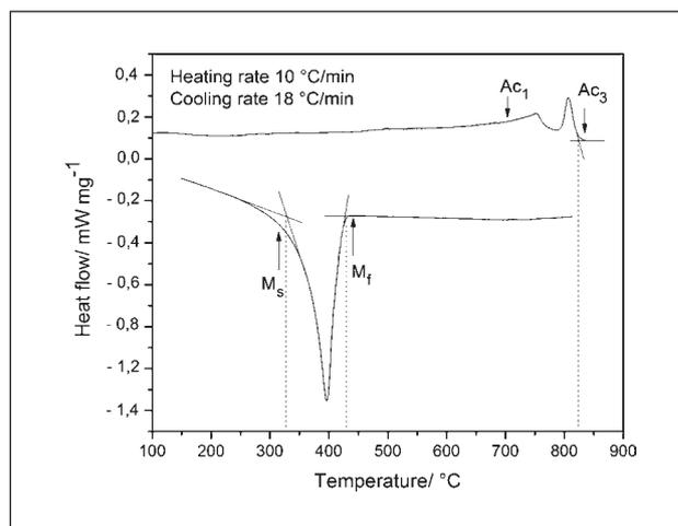
**Figure 2** DSC thermogram using a heating rate of 10 °C/min showing the transformation temperatures using intersection lines method.
