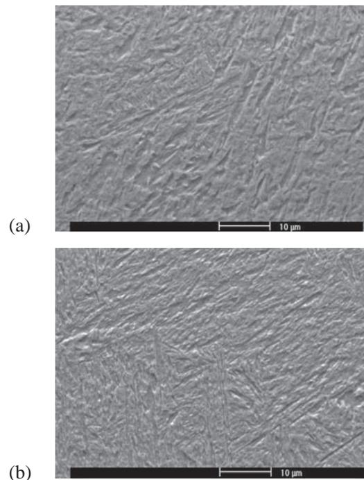
**Figure 6** Microstructure after dilatometric test;... (a) 60 °C/min, (b) 600 °C/min.
