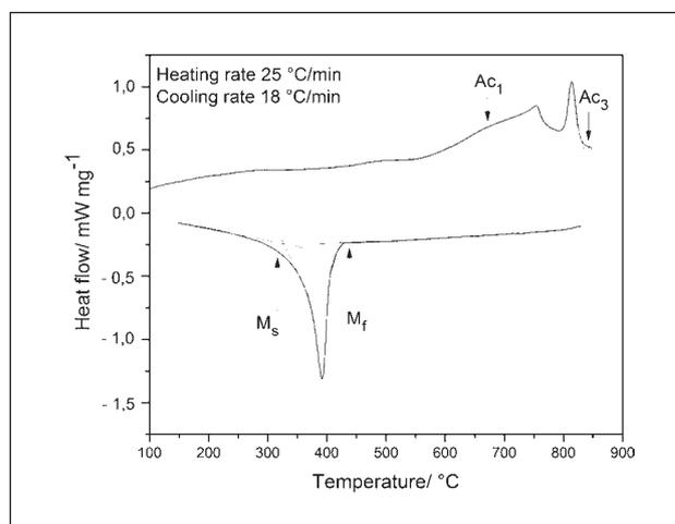
**Figure 3** DSC thermogram using a heating rate of 25 °C/min showing the transformation temperatures using intersection lines method.
