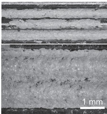
**Figure 11** (a) Gradual coating of W-wires  $d = 0,8$  mm with corundum ceramics, poor adhesion in the original, (b) improve adhesion to the  $WSi_2$  surface
