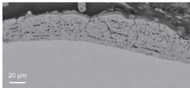
**Figure 3** Cross-section of tungsten wire with  $WSi_2$  coating
