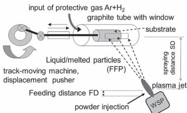
**Figure 5** Scheme of plasma spraying on movable or stationary tungsten substrates in a controlled atmosphere
