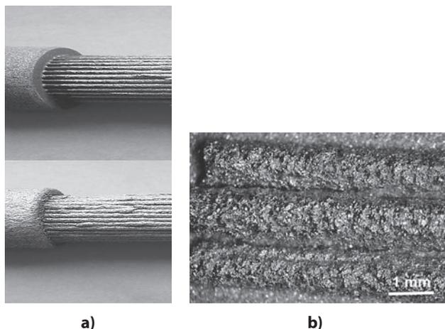
**Figure 6** (a) Deposition of tungsten on a complex armor wires and (b) the detail of the connection of individual wires
