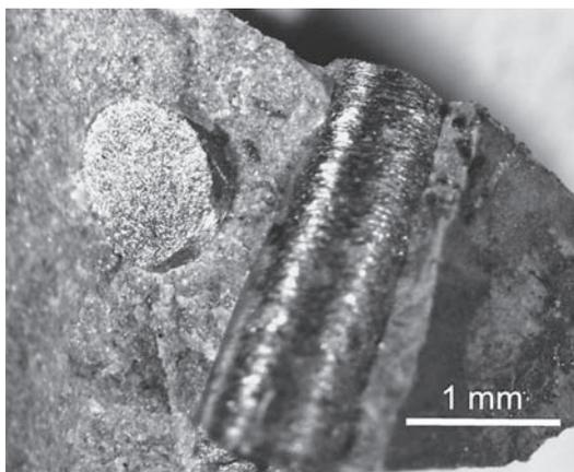
**Figure 10** Detail of the building of tungsten bars into a titanium matrix
