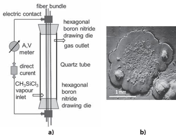
**Figure 1** (a) Scheme of SiC coatings preparation on a tungsten fibers and (b) the cross-section of the sheaf tungsten fibers in SiC matrix
