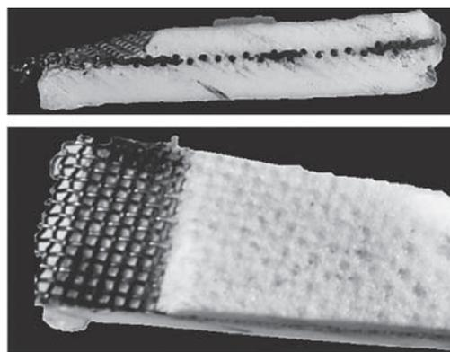
**Figure 9** Details of metal bars in the corundum matrix prepared by plasma spraying
