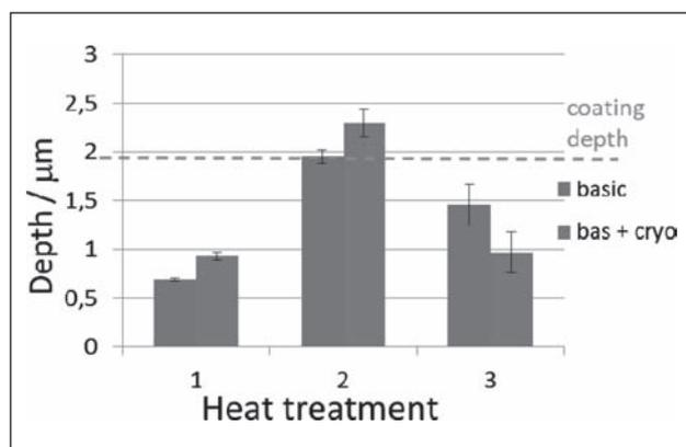
**Figure 1** Wear depth of a single layer TiAlN coating for different vacuum heat treated P/M steel substrates
