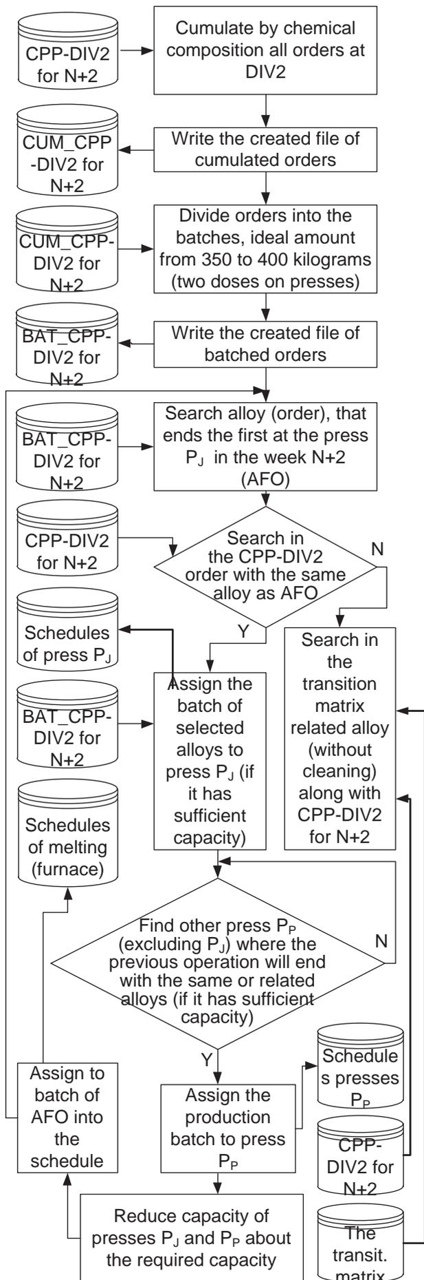
**Figure 4** Algorithm of the model of production scheduling creation at the section 2
