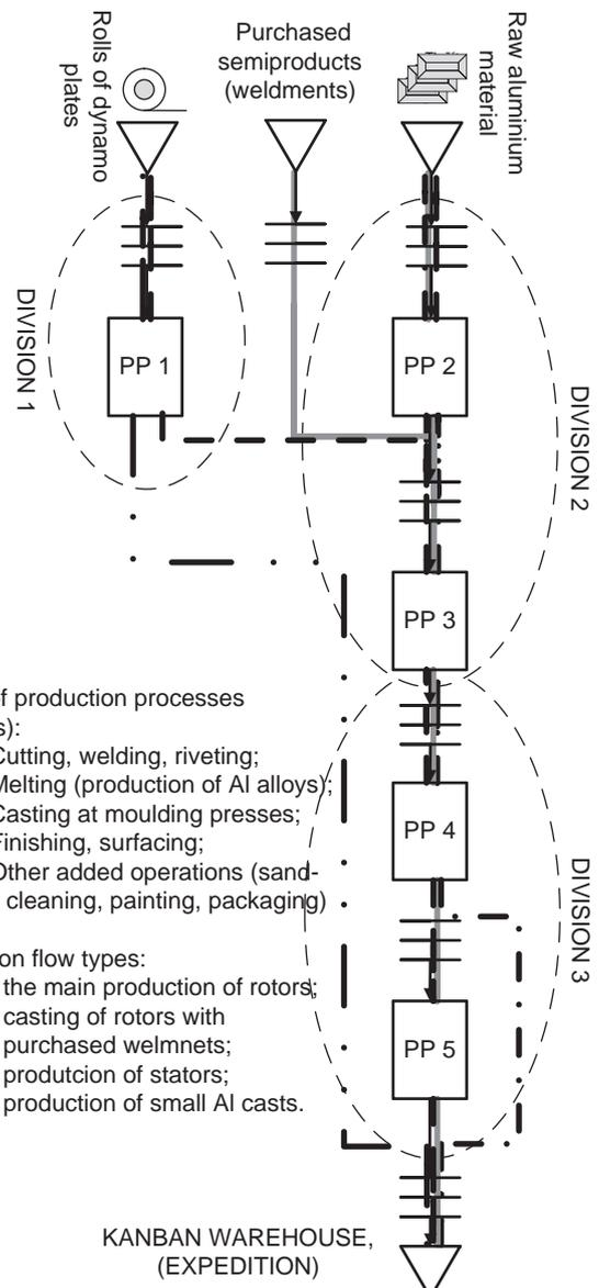
Figure 1 The manufacturing process – the block diagram [1]
