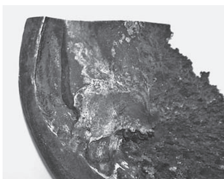
Figure 5 Detail of macro fracture
