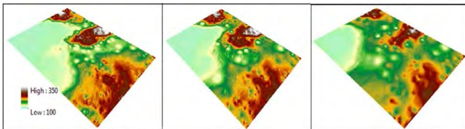
Fig. 4. DTM obtained by IDW interpolation (TK 25, TK50, TK100).
