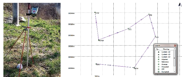
Figure 3 Marking of the FENO reference mark and the sketch of the geodetic support network
