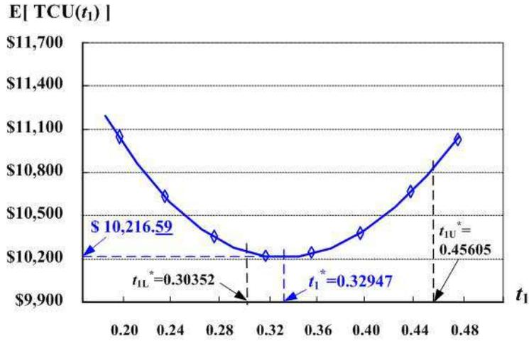
Fig. 3 The behavior of  $E[TCU(t_1)]$  with respect to production run time  $t_1$
