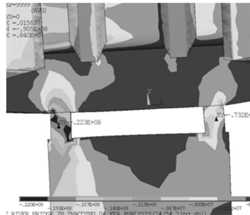
Fig. 4 Stress (50 %P + D+ A load)
