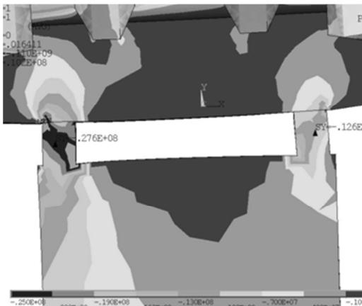
Fig. 3 Stress (100%P + D+A load)
