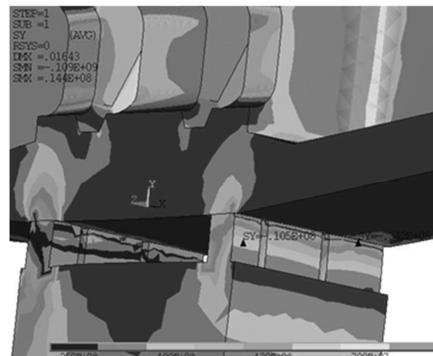
**Fig. 2** Temporary block vertical stress under dead + accidental load
