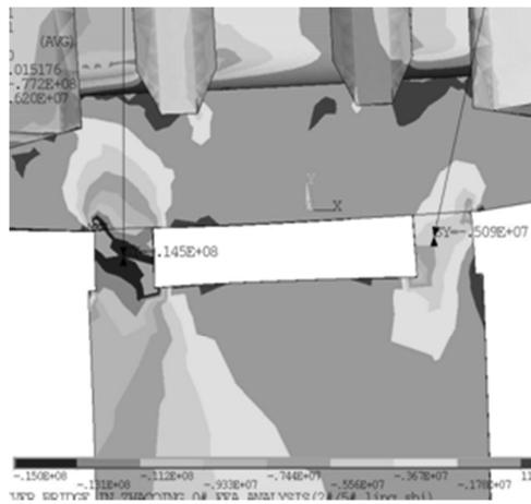
**Fig. 5** Stress (width=0.8 m 50%P+D+A)
