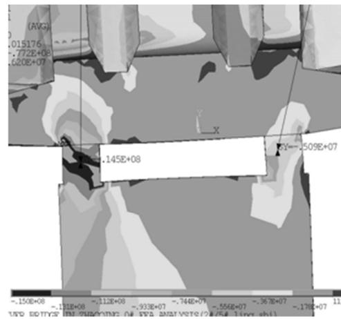
**Fig. 6** Stress (width=1.0 m 50%P+D+A)
