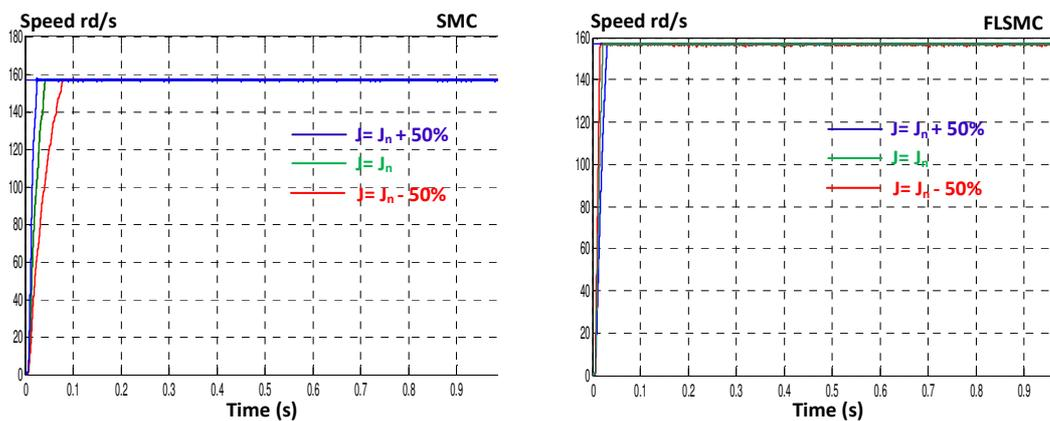
Fig. 8 Simulation results under variations of the moment of inertia
