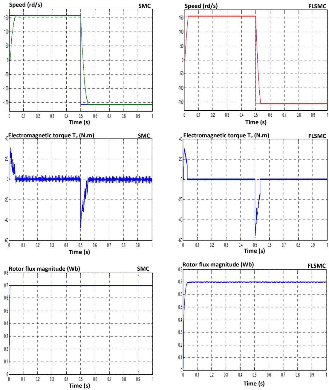
**Fig. 5** Comparison results between the SMC and FLSMC at no load  $T_L = 0$  N.m
