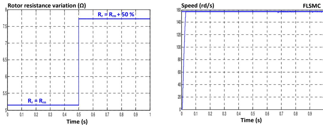
Fig. 7 Simulation results under rotor resistance variation
