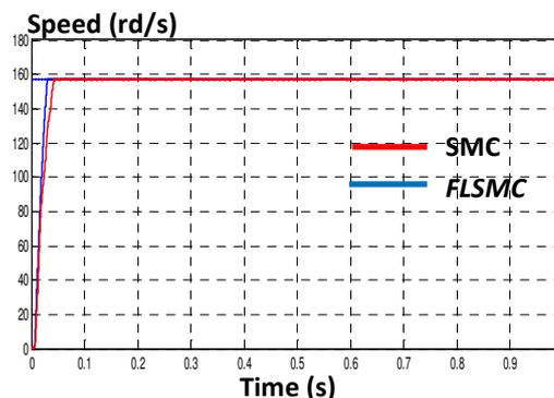
Fig. 4 Speed response comparison at no load  $T_L=0$
