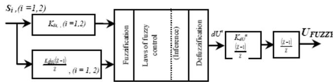
Fig. 1 Diagram of the fuzzy logic sliding mode controllers
