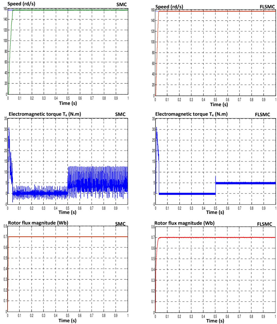
**Fig. 6** Comparison results between the SMC and FLSMC when load  $T_L = 5 \text{ N.m}$
