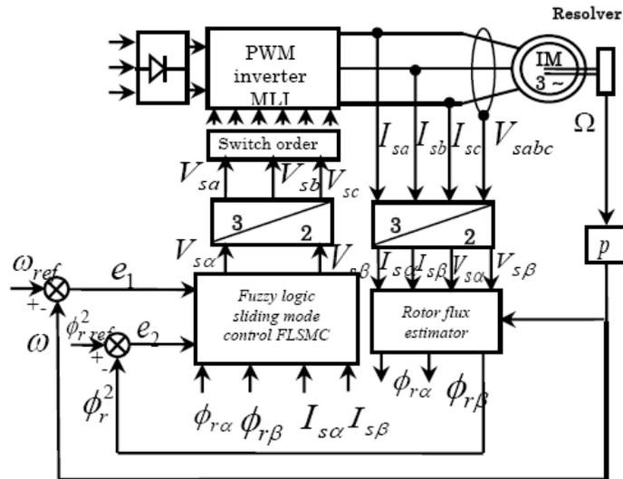
Fig. 3 Principle scheme of the proposed FLSMC of IM
