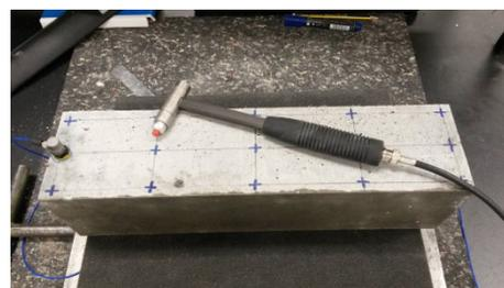
**Figure 2** Tested concrete specimen, accelerometer and impact hammer
