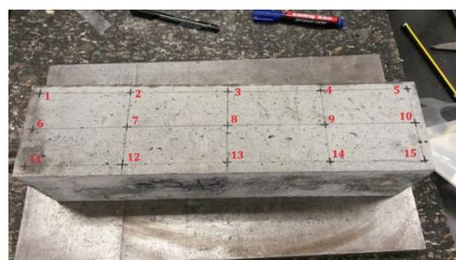
**Figure 3** Points being hit by impact hammer
