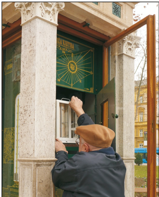
Fig. 2 Northern side of the post: Mr. Z. Lebarović returns the Lambrecht meteorograph at its place after the clock mechanism has been adjusted and thermo, baro and hygrograph paper replaced
