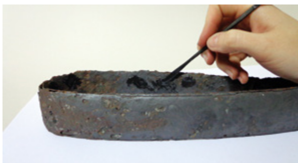
10. Ujednačavanje površine Aralditom 220 (fototeka HRZ-a, snimila E. Perković) Evening the surface with Araldite 220 (Croatian Conservation Institute Photo Archive, photo by E. Perković)
