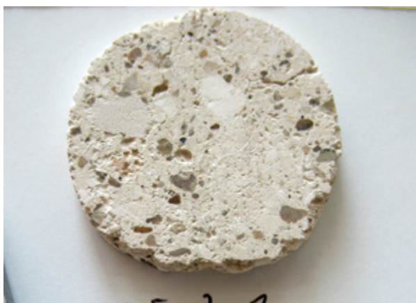
16. Standardizirani testni uzorak srednjovjekovnog arriccio (snimio B. Hacker, 2009.) Standardized test sample of the medieval arriccio (photo by B. Hacker, 2009)
