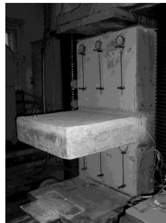
Figure 3. The general view of test sample, which is mounted on a press platform
