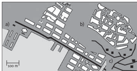
FIG. 7 RIJEKA – TYPES OF ROAD NETWORKS: A) ORTHOGONAL GRIDIRON, B) IRREGULAR MEDIEVAL, C) IRREGULAR TOPOGRAPHICAL
