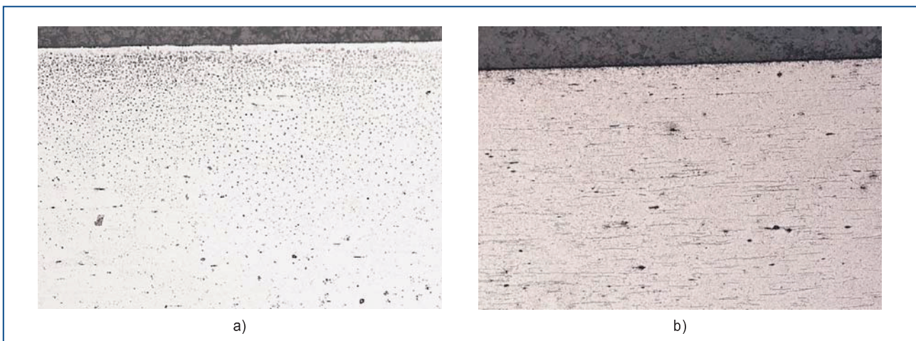
Slika 2. Mikrostruktura zakaljenih čelika, povećanje 200x: a) X20Cr13, b) X17CrNi16-2 Figure 2. Microstructure of hardened steel, magnification of 200x: a) X20Cr13, b) X17CrNi16-2
