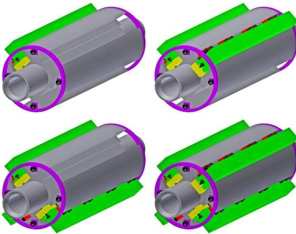
Figure 2. Scheme of preparation with 1 - 4 clamped slats [5].
