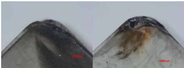
Figure 10. Wear of insert D210  $f = 0.2$  mm (left),  $f = 0.32$  mm; 4 slats [1].
