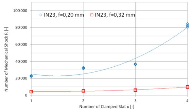
Figure 9. Dependence on number of shocks according to the number of the IN23 insert.
