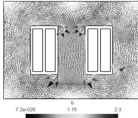
Figure 2. Transversal transformer cutaway: magnetic flux density distribution on the transformer core [25].
