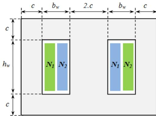
Figure 1. Transversal transformer cutaway: dimensions of the core, primary ( $N_1$ ) and secondary ( $N_2$ ) windings.
