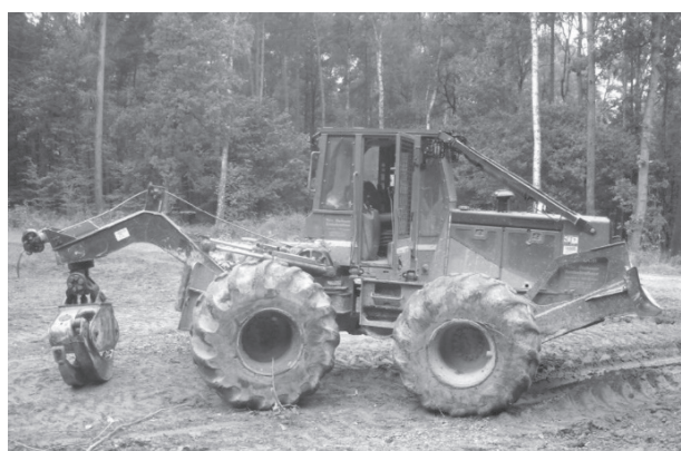
Fig. 1 Skidder equipped with a forest grapple observed during the investigations
