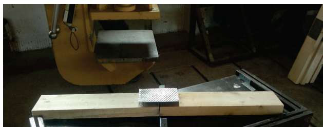
Figure 7 The embedding of the connector plate into the wood
