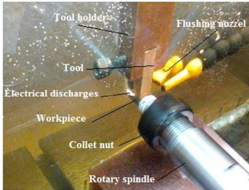
**Fig. 1** Concept of EDT process
