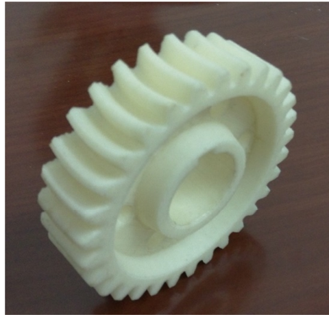
Fig. 11 CATT gear obtained by translational processing
