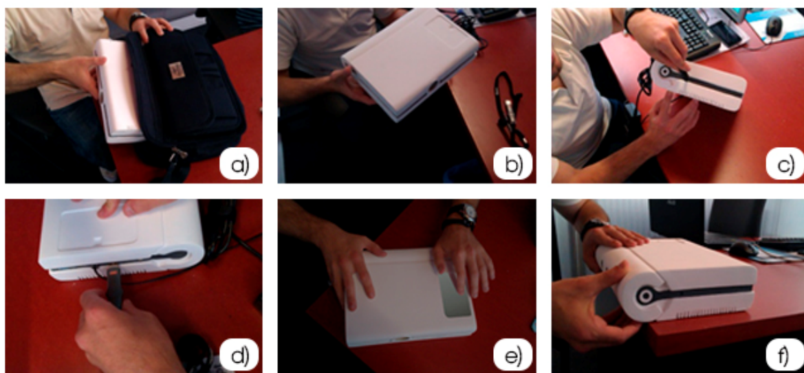
Fig. 15 Different phases of usability testing with users: a) Removing the device from the bag; b) Free observation and manipulation of the device; c) Connecting the device; d) Connecting the USB pen; e) Accessing the interface; f) Adjusting the position of the 3D sensor
