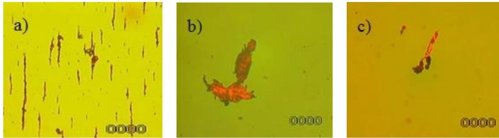
**Figure 4.** The demonstration of particles trapped onto the ferrograms of oil samples
