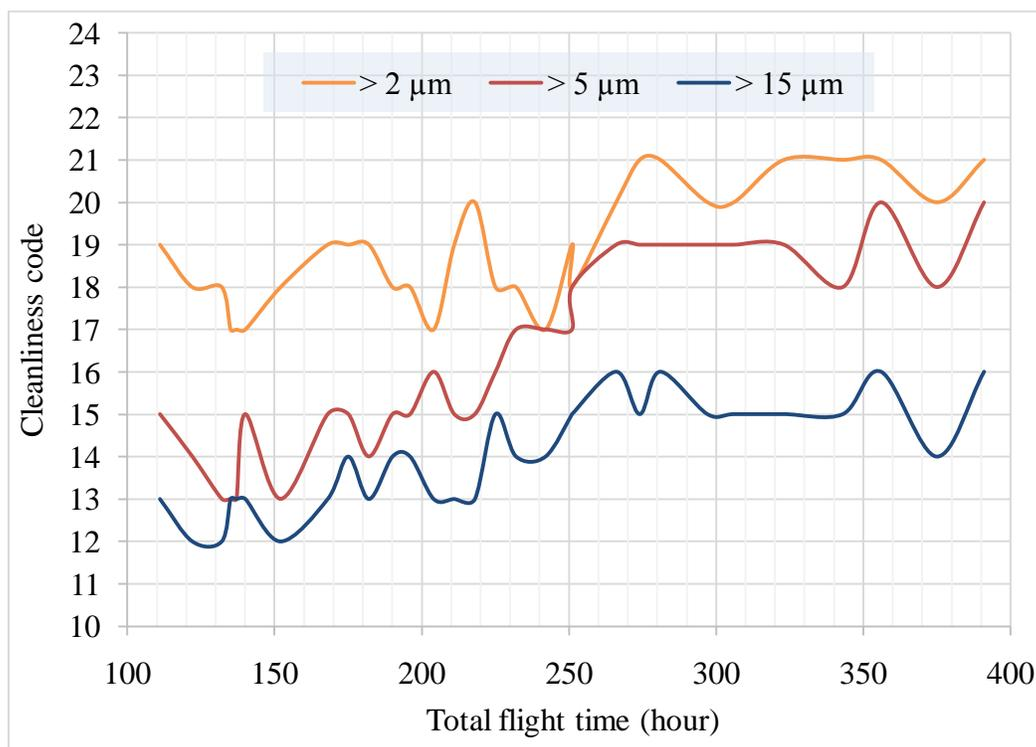
**Figure 3.** The course of changes in the cleanliness code of particles larger than 2  $\mu\text{m}$ , 5  $\mu\text{m}$  and 15  $\mu\text{m}$ , depending on the total flight time over approx. 300 hours
