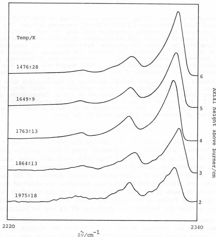
Figure 2. Stokes Raman spectra of nitrogen in methane-air flame,  $\Phi = 0.5$ , axial distance 2–6 cm above burner orifice. Radial distance 0 mm from burner axis.
