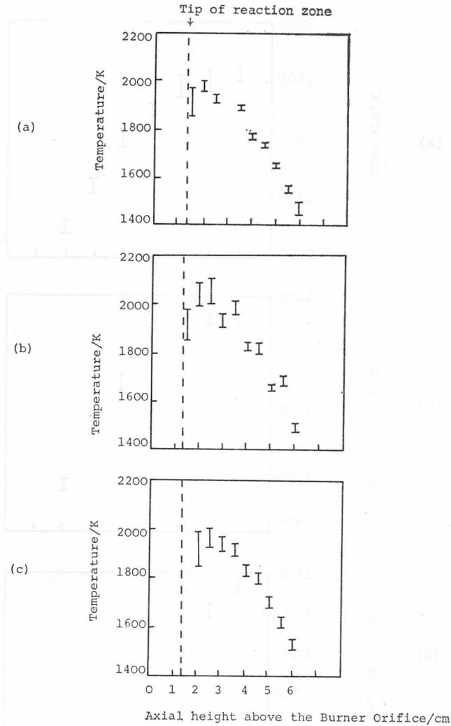
Figure 6. Axial temperature profiles of (a) methane-air, (b) propane-air, (c) butane-air flames, all  $\Phi = 0.5$ , for radial distance of 0 mm from the burner axis.
