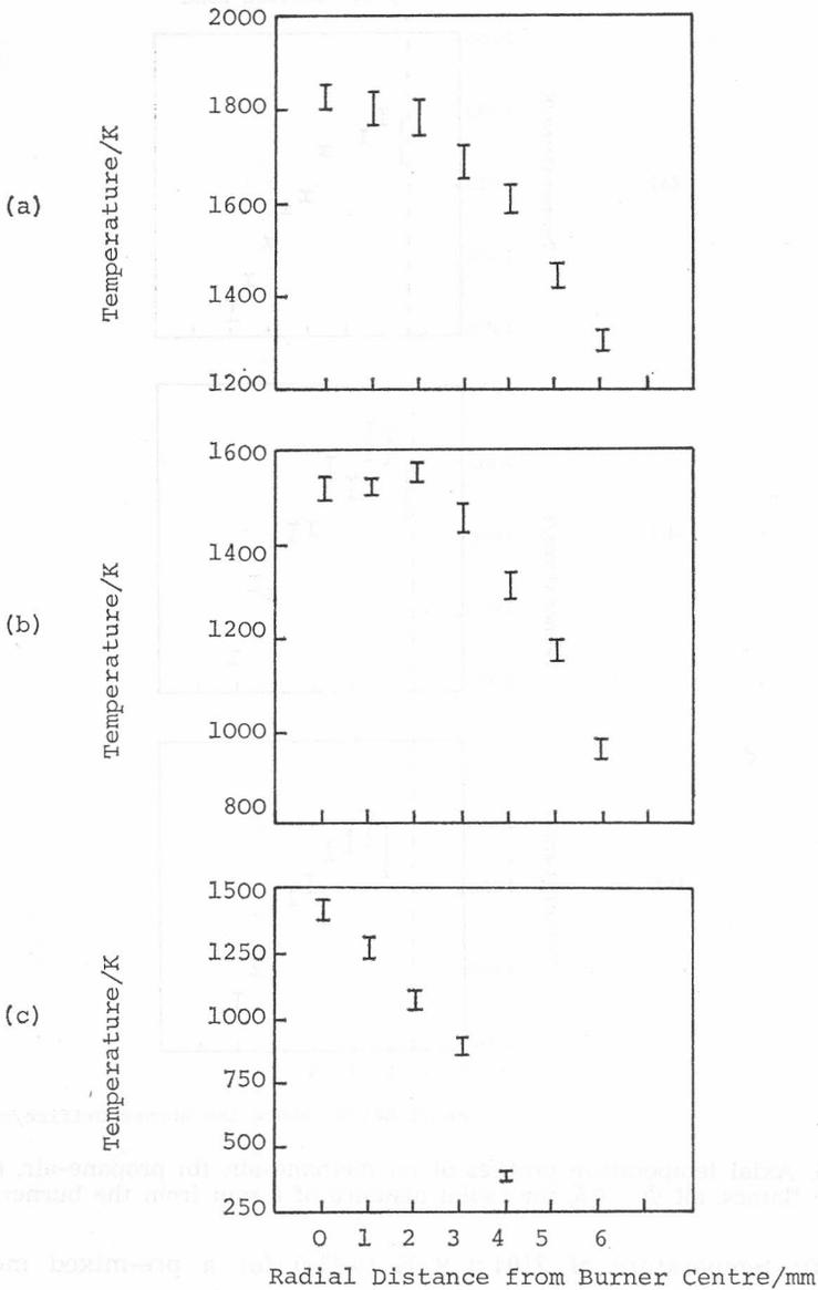
Figure 7. Radial temperature profiles in a butane-air flame,  $\Phi = 0.5$ , at axial heights of (a) 4 cm, (b) 6 cm, (c) 8 cm above the burner orifice.
