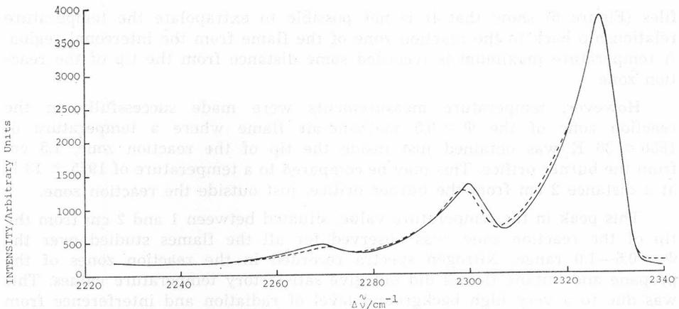
Figure 1. Unresolved Stokes Raman Q-branches,  $\Delta\nu = 2220\text{--}2340\text{ cm}^{-1}$ , for nitrogen in a methane-air flame,  $\Phi = 0.5$ , axial distance 5 cm above the burner orifice, radial distance 0 mm from burner axis. Observed spectrum —; computer fitted spectrum ----. Calculated temperature  $T = 1571 \pm 9\text{ K}$ . Observed spectra collected in 256 channels.
