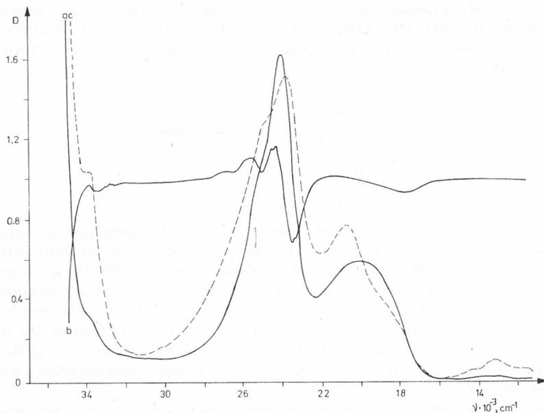
Figure 2. Reversible temperature variations of the electron absorbance spectrum of  $AS^-$ - $AHQ^-$ ; a) 25 °C,  $\lambda_{max}$  (lg  $\epsilon$ ); 262 (4.27), 416 (3.96), 499 (3.51), 746 (1.82) nm; b) 25 °C, first derivative of the spectrum; c) 96 °C,  $\lambda_{max}$  (lg  $\epsilon$ ); 262 (3.97), 282 (4.15), 420 (3.91), 480 (3.62), 756 (2.73) nm. Evacuated cuvette,  $1.86 \cdot 10^{-4}$  M solution of 1 in 1 M aqueous NaOH.
