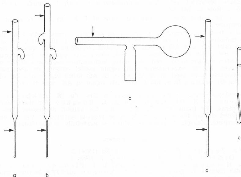
Figure 4. Vessels used in measurements: a) 1 only, ESR; b) 1 with lignin models, ESR; c) 1 only, electron absorbance; d) AQ with wood extract and various organic compounds, ESR; e) the latter in microthermostat with paraffin oil. Arrows indicate the places of sealing.
