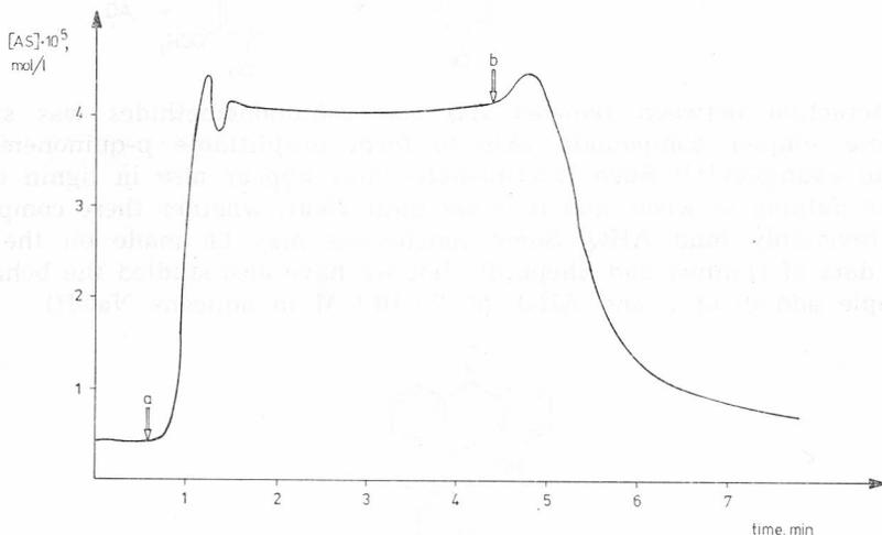
Figure 3. Typical kinetic cycle of reversible temperature variations of the  $AS^-$  concentration. The arrows indicate moments of sample temperature rise (a) from 25 to 170 °C and decrease (b) from 170 to 25 °C. Evacuated ampule, AQ (1 mg) in 0.01 ml of 1 M aqueous NaOH extract of spruce chips; ESR technique.
