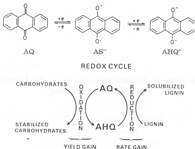
Figure 1. A redox cycle proposal for explaining the catalytic action of AQ during alkaline wood pulping.<sup>2</sup>
